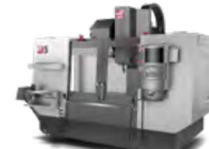
VF-5 40/50 TAPER • Travels 1,270 x 660 x 635 mm • 8,100 rpm 40-Taper • 30 hp • 20 Tool Carousel (SMTC option) • 7,500 rpm 50-Taper • 30+1 SMTC standard on 50-taper
