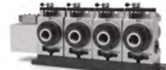
HA5C4 4-AXIS • Torque 34 Nm • 200°/sec • Resolution 0.001°
