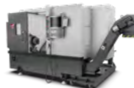
ST-20 • Max Cut Ø 330 x L 572 mm • Bar Capacity 64 mm • A2-6 • 4,000 rpm • 20 hp • Chuck 210 mm
