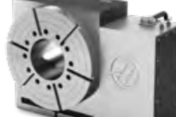
HRT630 4-AXIS • 630 mm Platter • 50°/sec • Resolution 0.001°
