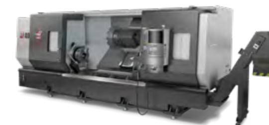
ST-40 • Max Cut Ø 648 x L 1,118 mm • Bar Capacity 102 mm • A2-8 • 2,400 rpm • 40 hp (55 hp opt.) • Chuck 381 mm
