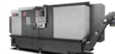
ST-30L LONG BED • Max Cut Ø 381 x L 1,588 mm • Bar Capacity 76 mm • A2-6 • 3,400 rpm • 30 hp • Chuck 254 mm
