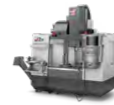
VF-2YT EXTENDED Y-AXIS • Travels 762 x 508 x 508 mm • 8,100 rpm • 40-Taper • 30 hp • 20 Tool Carousel Changer • (SMTC optional)
