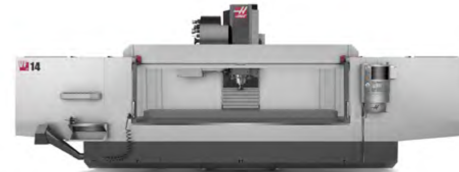
VF-11 40/50 TAPER • Travels 3,048 x 1,016 x 762 mm • 8,100 rpm 40-Taper • 30 hp • 7,500 rpm 50-Taper • 30 hp • 30+1 Side-Mount Tool Changer
