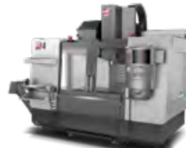
VF-4 • Travels 1,270 x 508 x 635 mm • 8,100 rpm • 40-Taper • 30 hp • 20 Tool Carousel Changer • (SMTC optional)
