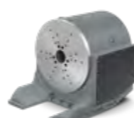
TH450 4-AXIS THROUGH HOLE • 450 mm Platter • 75°/sec • 82.55 mm Through-hole • Resolution 0.001°
